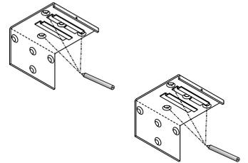
Place the mounting brackets at the desired height on the wall or ceiling and mark the holes for the dowels (see fig.). Drill holes and insert dowels.
