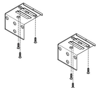
Place the mounting brackets on the wall or ceiling and fasten them lightly with screws. Align the brackets in a horizontal position. Tighten the screws.
